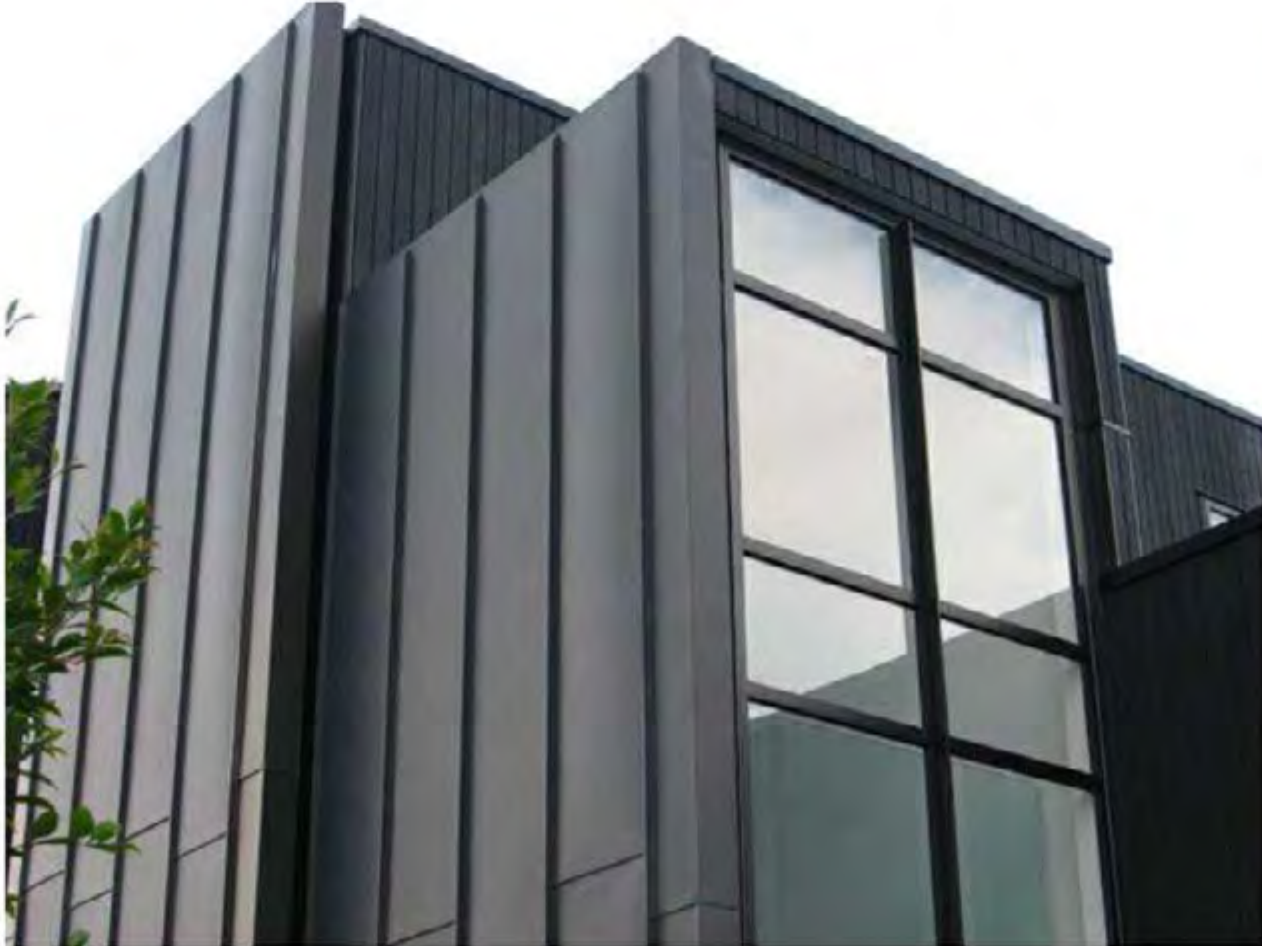
Dark zinc cladding • Streamlines building and aesthetic • Attractive contrast against brick
